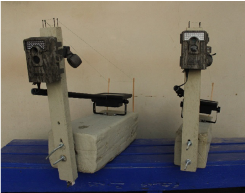
Completed mountings for time lapse cameras are ready to be installed in the field.
